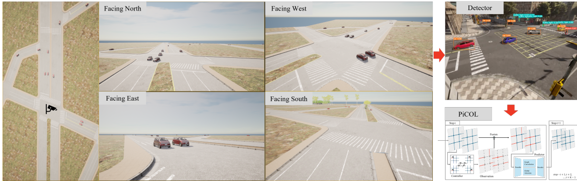
Figure 13: Cyber-Physical world implementation using CARLA-SUMO Co-simulation framework based on Flatbush corridor's network.
