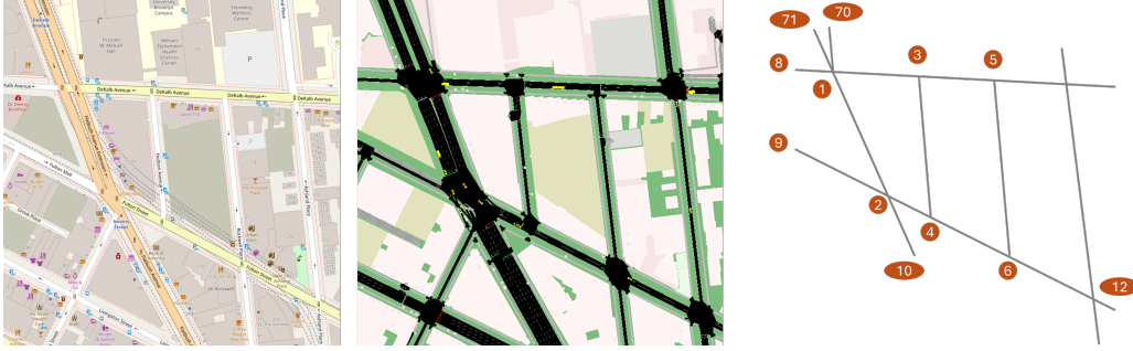
Figure 6: The simulation network building process. Left to right: Open Street Map, Network in SUMO, Abstracted Network.
